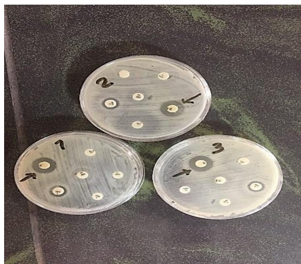
Figure 2: Formation of a halo of ingrowth in the disk diffusion test
