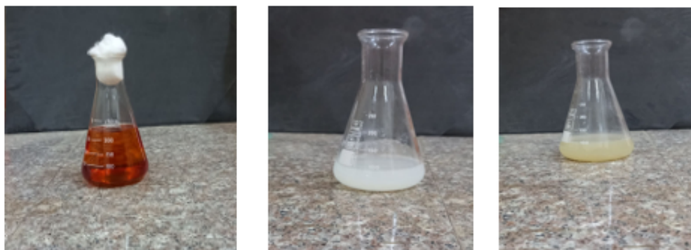
Figure 5. A B C Figure (3-1): Color transformation of the zinc oxide solution due to the effect of the plant extract. (A) P. farcta fruit extract solution. (B) Zinc oxide solution before adding the extract. (C) Zinc oxide solution after adding the extract.
