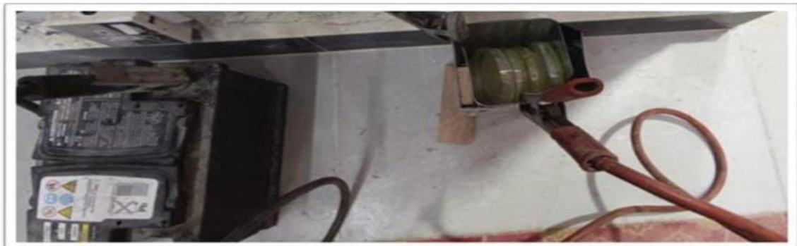
Figure 1 The application of an electric field on bacteria for 60 minutes using 60 A battery
